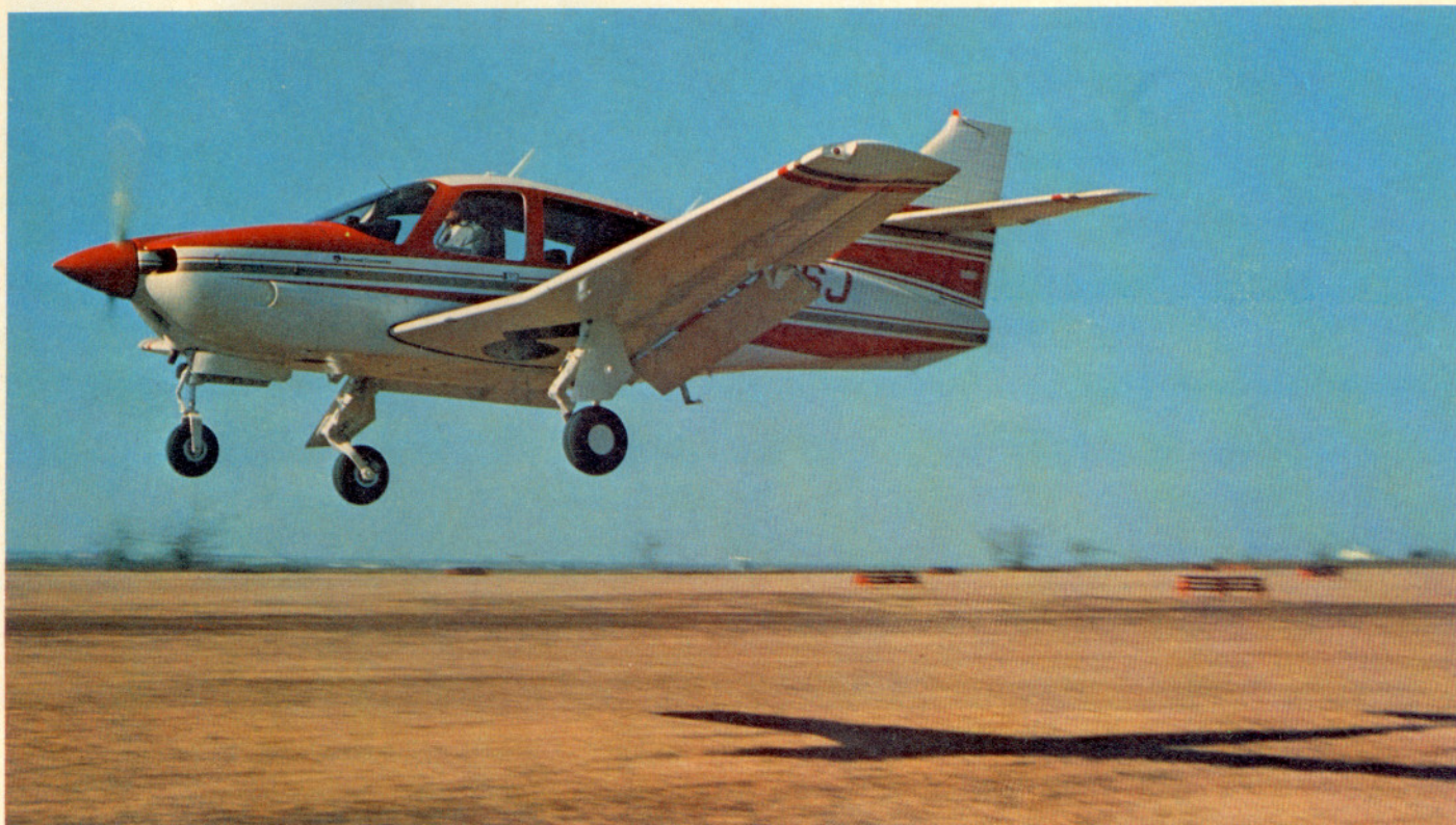
With wheels down, the 112A's trailing-beam main gear shock absorber system can be seen.
